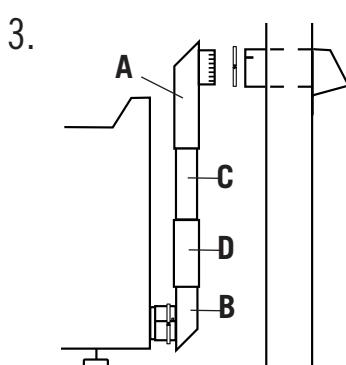
If both periscope fittings need to face to the front, refer to "Facing fittings to the front" section.
