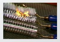
Crushed venting is one of the most common causes of dryer fires and maintenance calls.
