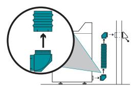
Crimped fittings are designed to Snap-Lock™ to elbows (like the Close Elbow™pictured). The soft-cuff slotted end will fit over most 4" connections and compress down for a secure fit.
