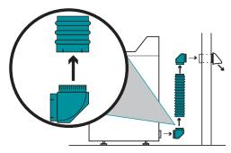
Builder's Best® Flexible pipe is designed to Snap-Lock™ to elbows (like the Close Elbow<sup>™</sup>pictured) or to other pieces of V830 for longer runs
