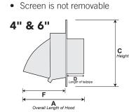
• UV stabilized polymer resin • Drip edge to help drain away water
